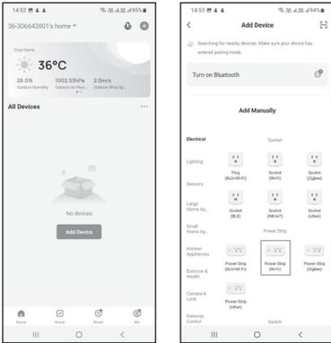
6. Make sure your smartphone and WiFi socket are on the same 2.4G WiFi network. The connection process takes about 30-120 seconds, depending on the state of the network and the length of the WiFi password.
